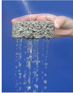
Pervious Concrete allows Groundwater Recharge.
